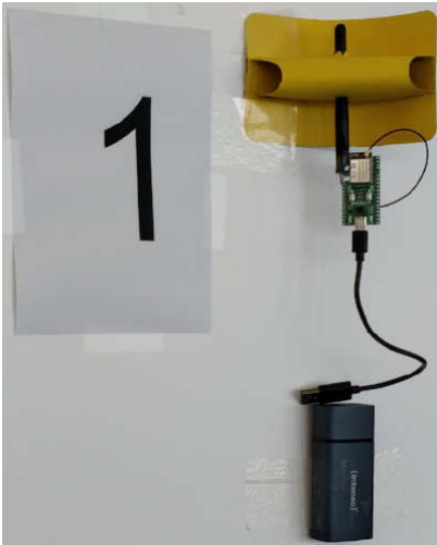
Fig. 3. ESP32 microcontroller with antenna, curved signal reflector, and powerbank.
